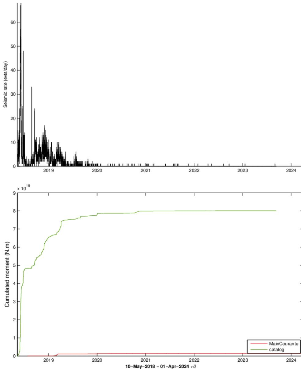
Instantaneous seismic rate (144.0/day samples) calculated on a moving, 24h fixed-size, time window
